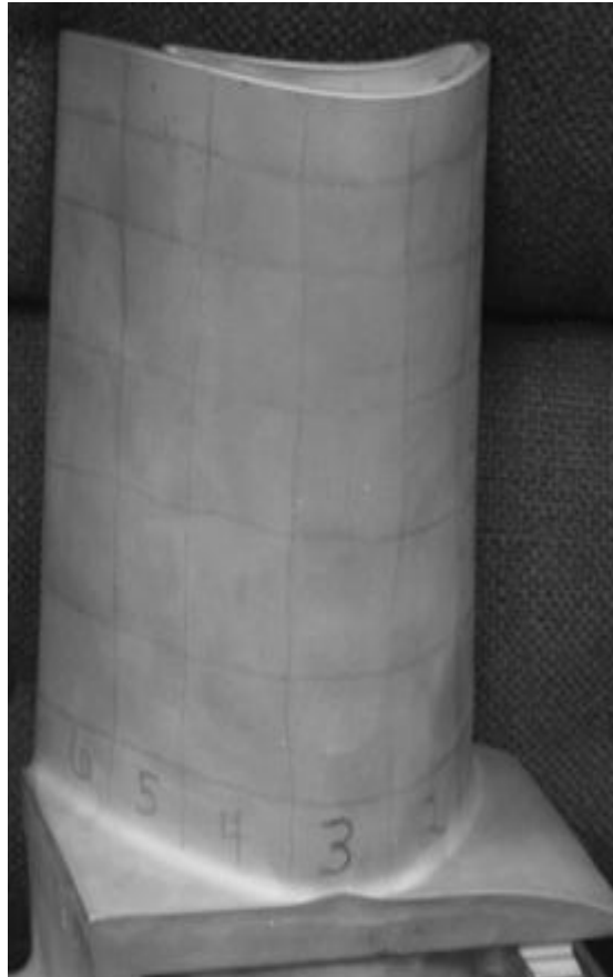
Figure 3: Showing a section of an actual turbine blade. The suction side faces the viewer, with the leading edge to the right. The chord length is measured along the suction side from the leading edge to the trailing edge.
